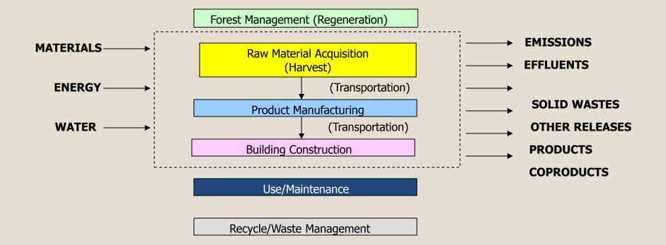
This analysis could be conducted as shown above, with consideration given to forest harvesting (but not forest restoration), production and transport of building materials, and all aspects of building construction. Use/maintenance and end-of-building-life are not included.
