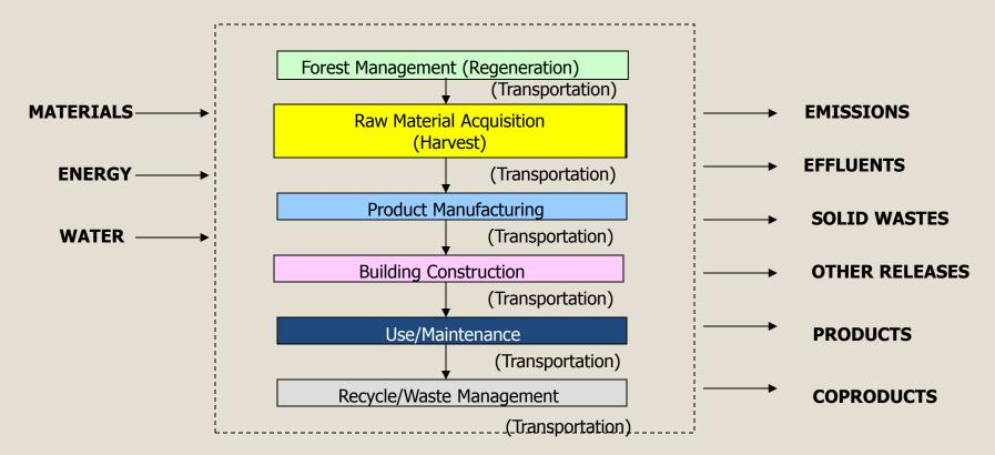
The dashed line above defines the system boundary for this analysis, defining what is to be considered. In this case, all steps in building materials production, transport, building construction, use and maintenance, and deconstruction or demolition are included.
