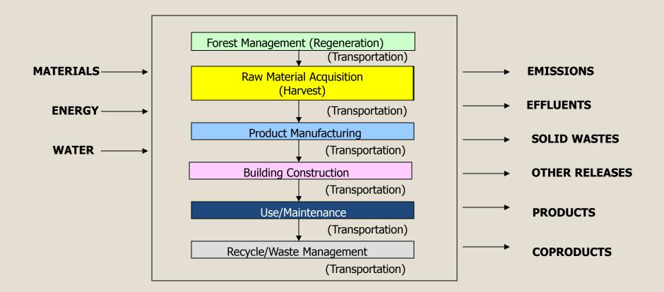
Conceptually, an LCI looks like this. In this case a wood building is analyzed beginning with raw material extraction through end of building life, with all inputs and outputs considered.
